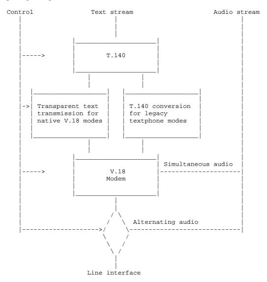
Figure : Text telephone package functional view
