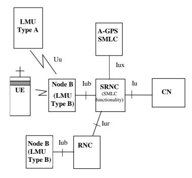
The new interface will need to support two types of messages; service invocation messages and positioning messages. The service invocation messages can be based on the Lb interface as defined in GSM 09.31 and GSM 08.71. The service invocation messages will provide for a request/response message exchange such that the SRNC can query the SMLC for the position of the UE.
