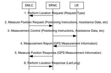
In the case of incomplete assistance data in the "measurement command", RRC allows for an UP error message to be returned to the SRNC with an explicit request for assistance data that will be provided to the SMLC. This would result in the steps 2 though 5 being repeated.
