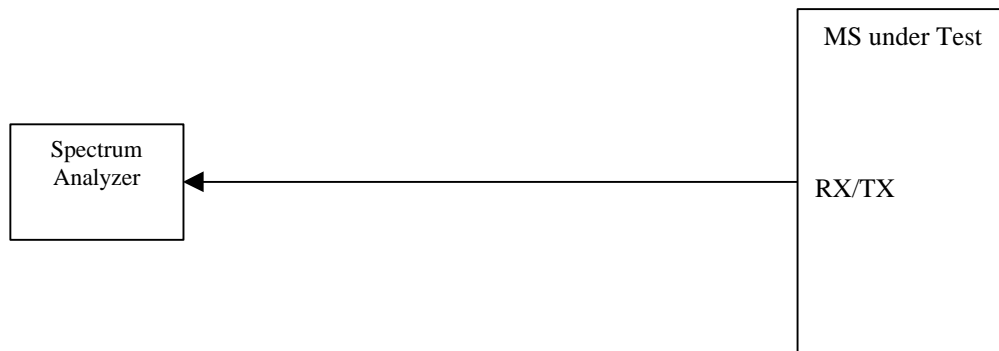
Figure A.8 Connection for Spurious Emission Test
