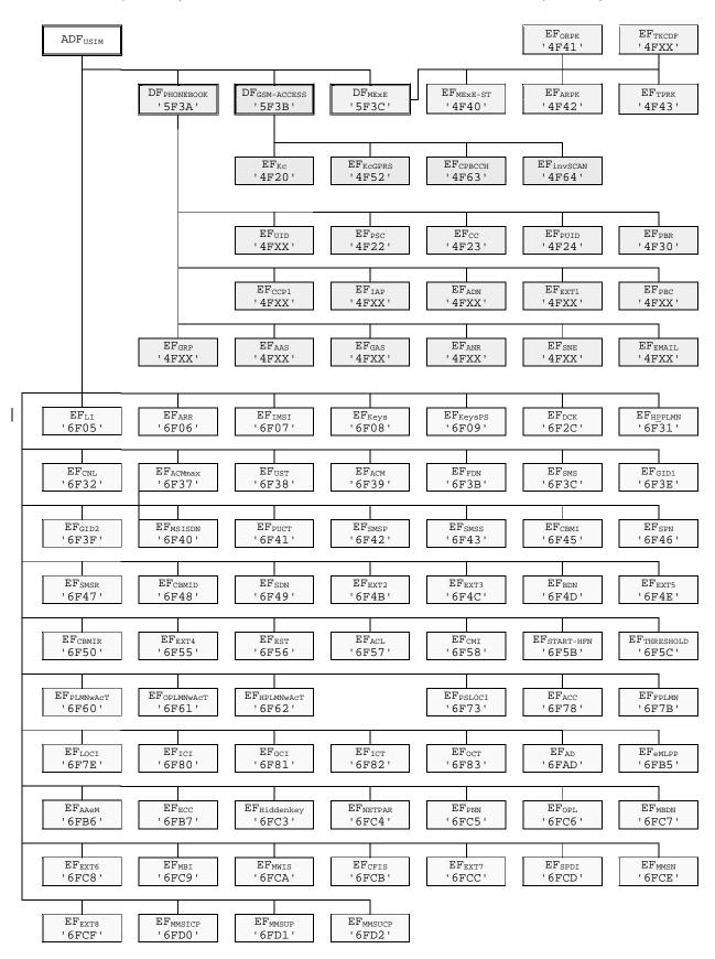
Figure 4.2: File identifiers and directory structures of USIM
