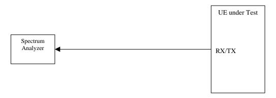
Figure A.8: Connection for Spurious Emission Test
