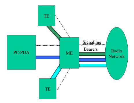
The above diagram illustrates an ME connected to a radio network with different TE devices requiring different bearer and signalling capabilities from the ME.
