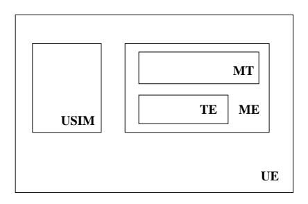
The figure below shows an example of a physical configuration of a UE.
