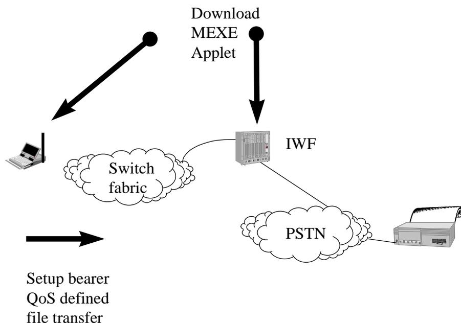
This permits an advanced terminal in a UMTS or enhanced GSM network to communicate with a fax machine in the PSTN using MEXE to define the functionality at the mobile terminal and the network equivalent (sometimes called NEXE) to define the functionality in the interworking function. Upgrades to hardware are not required given that the support of the execution environment is available.
