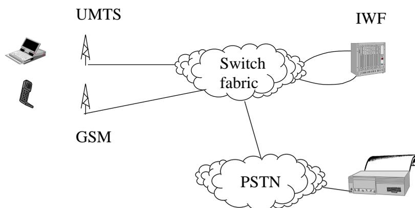
In this context, full handover means that the call can be initiated either on the GSM or the UMTS network and if coverage of one of the networks disappears during a call then the call is handed to the other technology. Handover between cells on the same technology is also assumed.
