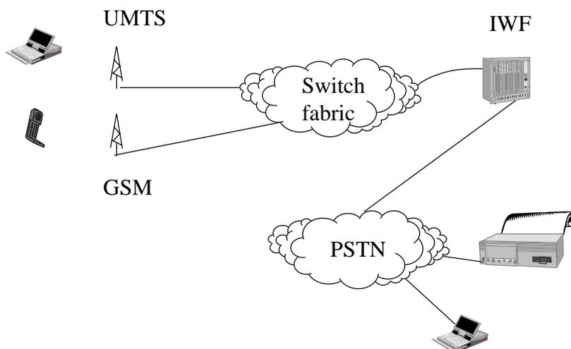
The IWF provides a range of modems which can be accessed via a circuit switched or packet switched connection. These modems could talk over the PSTN to other modems or to fax machines, entirely at the discretion of the caller. The caller would first establish a connection to the modem and the instruct the modem as to how to set the call up from there. When the call is disconnected then a message is sent back to the user advising of the call cost.
