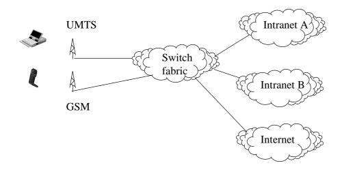
This scenario shows how connections can be established to the Internet or Intranets, following the GPRS model.
