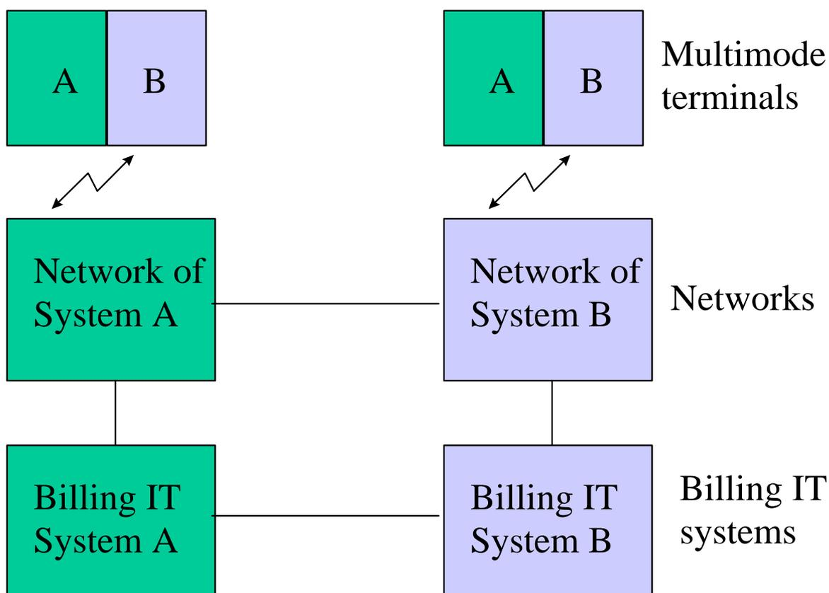
**Figure 1: Architecture for Inter System Roaming**
