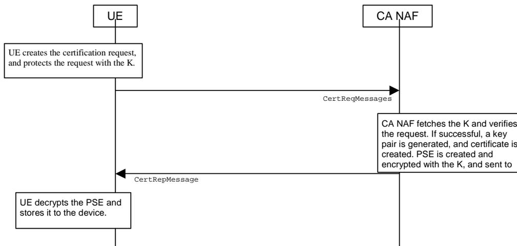
**Figure 3: Certificate request using centralized scheme of CMP.**
