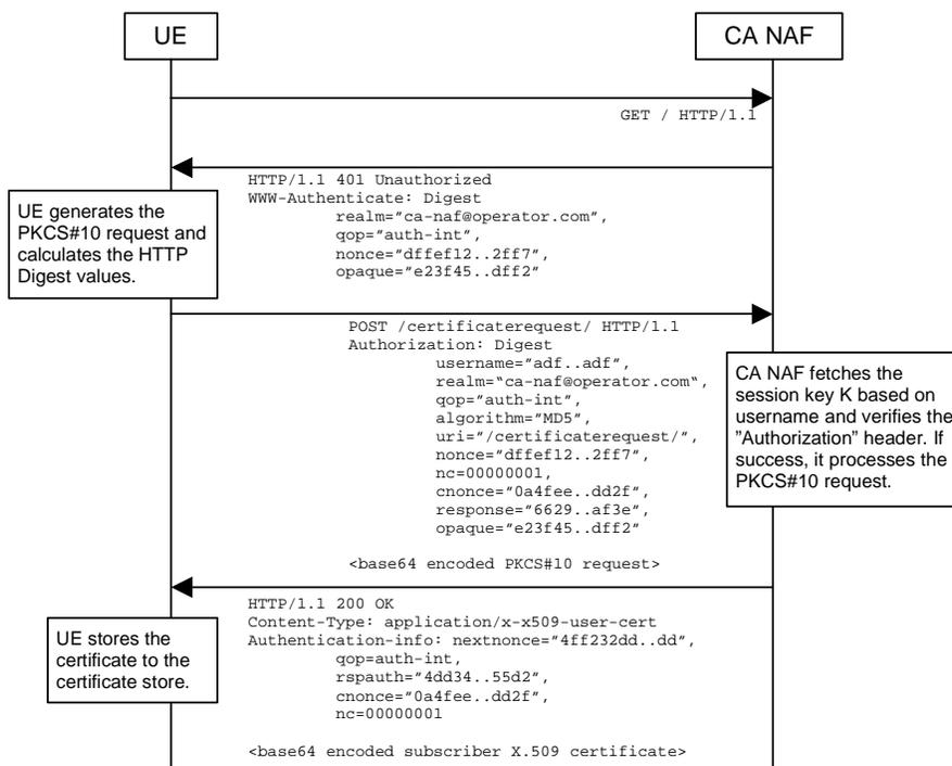
**Figure 1: Certificate request using PKCS#10 with HTTP Digest Authentication.**
