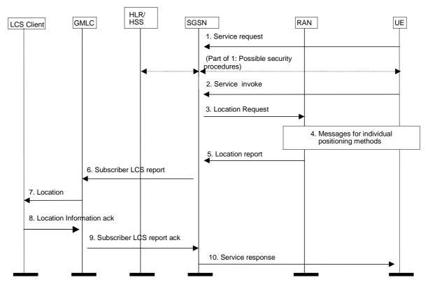
Figure 9.8: General Network Positioning for packet switched MO-LR
