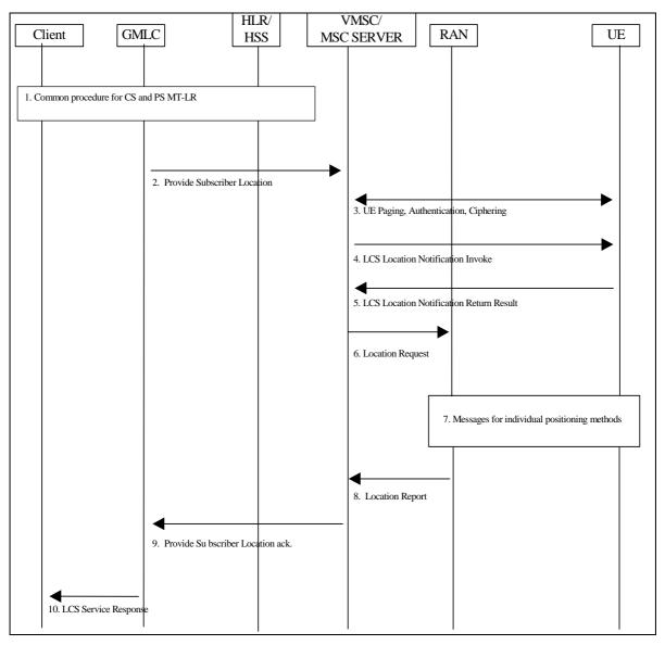
Figure 9.2: Network Positioning for a CS-MT-LR
