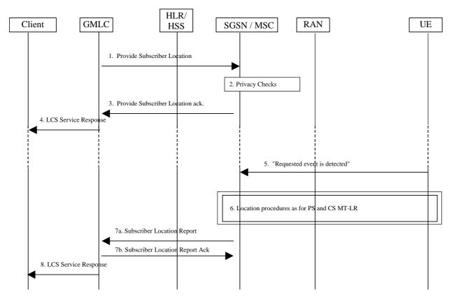
Figure 9.6a: General Network Positioning for a Deferred MT-LR
