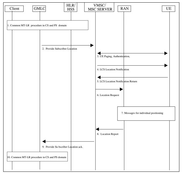
Figure 9.2: Network Positioning for a CS-MT-LR
