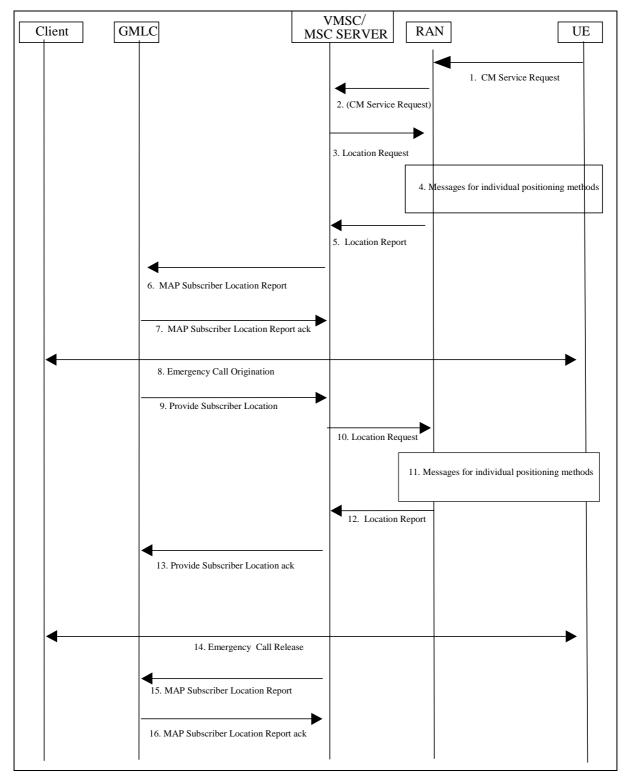
Figure 9.4A: Positioning for a NI-LR Emergency Service Call using Location Based Routing
