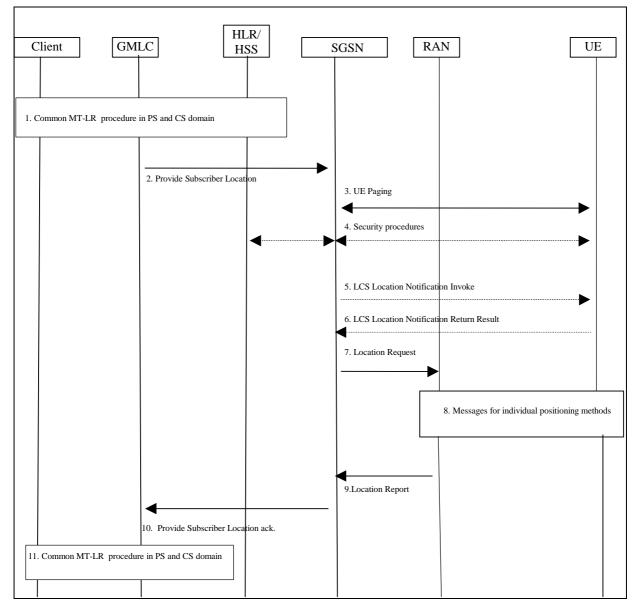
Figure 9.5: General Network Positioning for Packet Switched MT-LR
