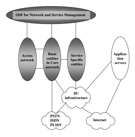
Figure 7.4: High level <u>3GPP system UMTS</u> Network architecture
