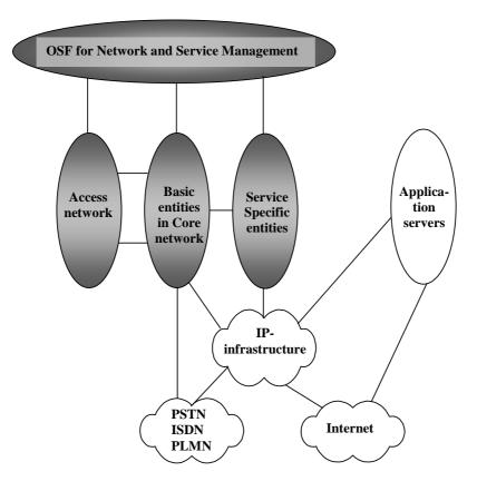
Figure 7.4: High level 3GPP systemUMTS Network architecture
