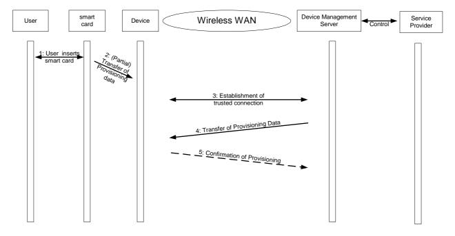
Smart Card based Provisioning including a partial transfer of provisioning data (Normal Flow)
