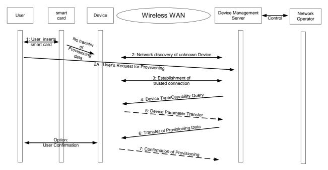
Provisioning for used Devices including network detection (Normal Flow)
