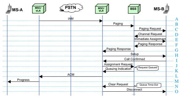
Figure 5.8 Priority Service Mobile Terminated – Queue Time-Out
