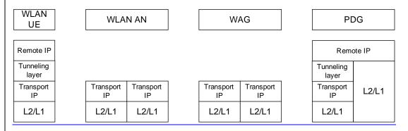
Figure 6.3. Protocol stack between the WLAN UE and the Packet Data Gateway
