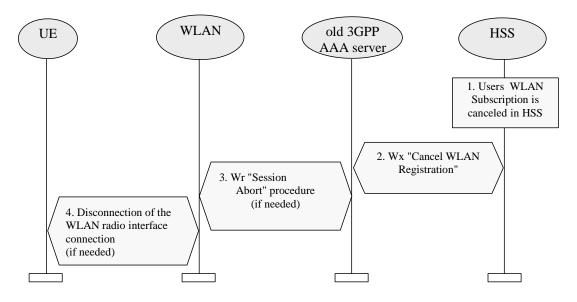
Figure 7.3 Cancellation of WLAN Registration Procedure
