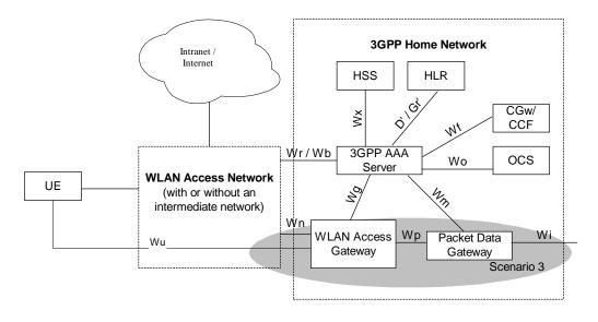
Figure E.1.1 Non Roaming Reference Model
