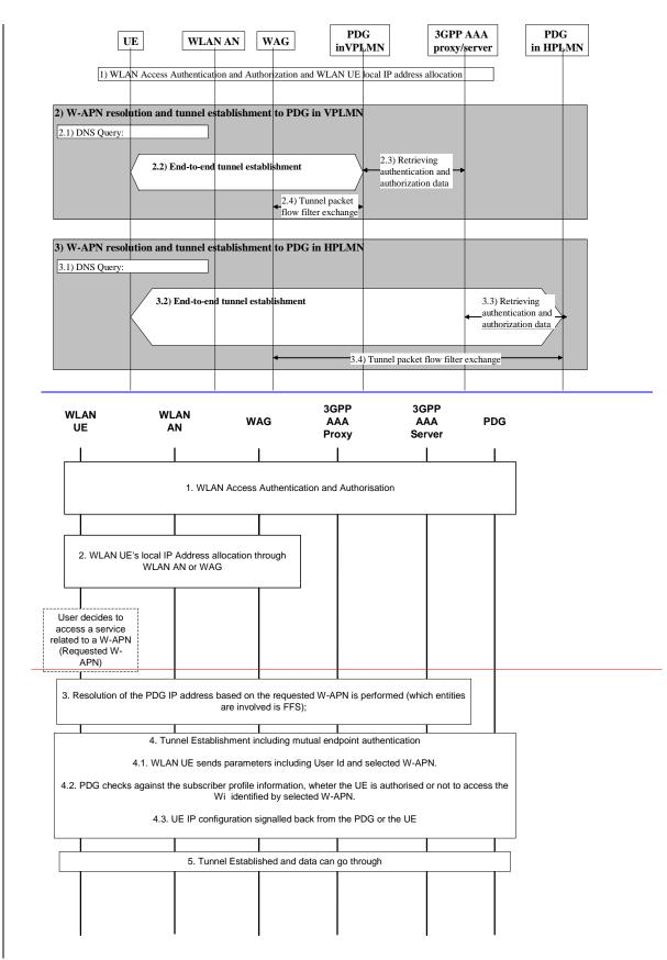
Figure 7.8. Example message flow to WLAN UE-Initiated tunnel establishment
