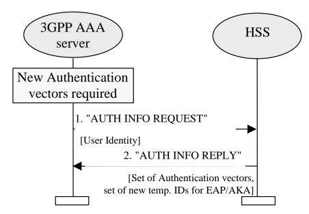
Figure A.2.1 Signalling example on Wx Reference Point for Authentication Information Retrieval
