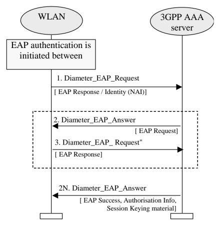
Figure A.1.1 Signalling example on Wr Reference Point for Authentication and Authorisation
