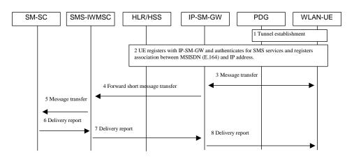
Figure D.3: SMS origination from IP terminal
