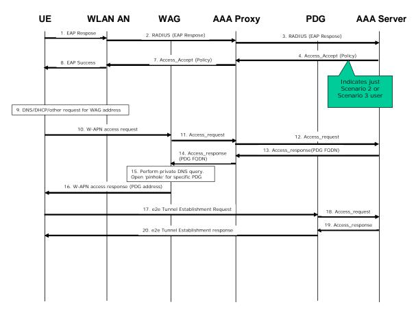
Figure F.1.2 - WAG DNS client based W-APN resolution
