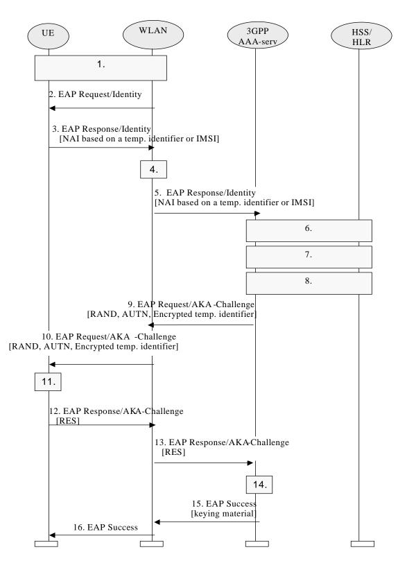
Figure A.5.1 Authentication based on EAP AKA scheme
