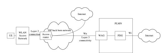
Figure C.4.1 Wn Interface when WLAN is connected to a PLMN through an ISP
