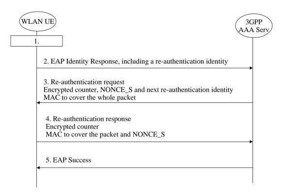
Figure A.4.4 Re-authentication signalling sequence
