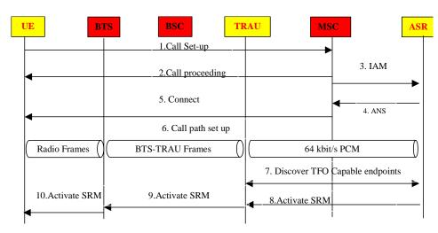
Fig.1 TFO Signalling Flows between GSM Terminal and ASR Unit
