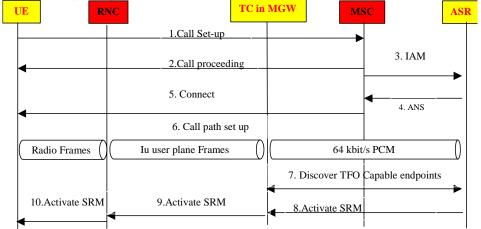
Fig.2 TFO Signalling Flows between UMTS Terminal and ASR Unit
