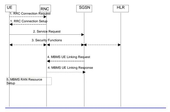
Figure x: MBMS Service Request procedure
