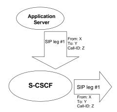
Figure 4.3b: Application Server acting as originating UA
