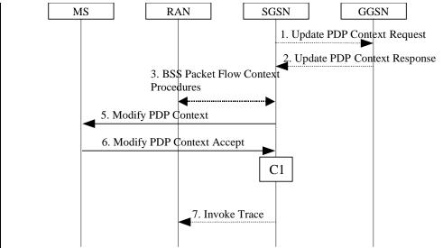
Figure 70a: SGSN-Initiated PDP Context Modification Procedure, A/Gb mode
