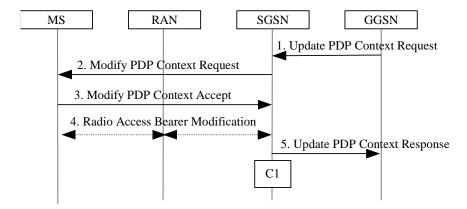
Figure 71: GGSN-Initiated PDP Context Modification Procedure
