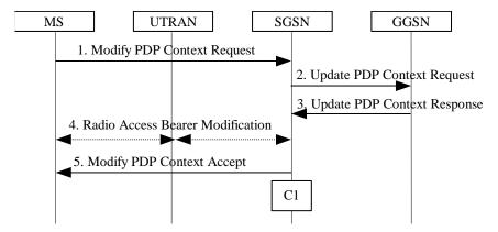
Figure 7: MS-Initiated PDP Context Modification Procedure
