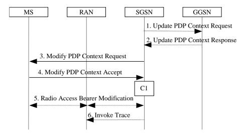
Figure 70: SGSN-Initiated PDP Context Modification Procedure
