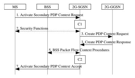
Figure 65: Secondary PDP Context Activation Procedure for GSM
