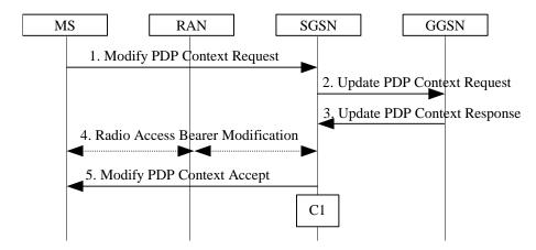
Figure 72: MS-Initiated PDP Context Modification Procedure
