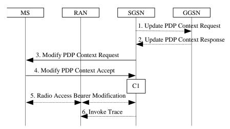
Figure 70: SGSN-Initiated PDP Context Modification Procedure
