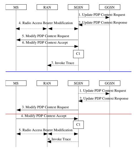
Figure 70b: SGSN-Initiated PDP Context Modification Procedure, lu mode
