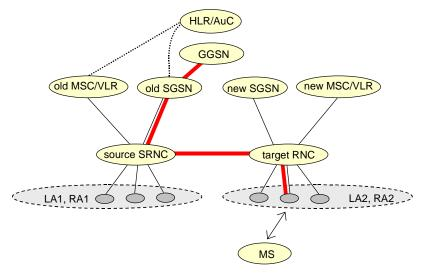
Figure 37: Before SRNS Relocation and Routeing Area Update
