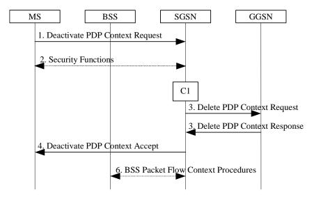
Figure 74: MS Initiated PDP Context Deactivation Procedure for A/Gb mode
