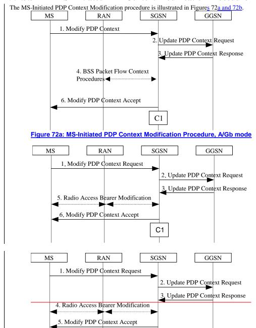
Figure 72b: MS-Initiated PDP Context Modification Procedure, lu mode
