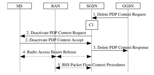
Figure 77: GGSN-initiated PDP Context Deactivation Procedure
