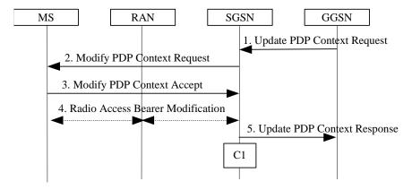
Figure 71: GGSN-Initiated PDP Context Modification Procedure
