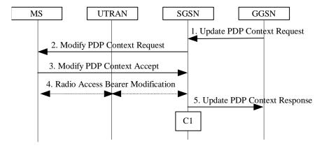
Figure 71: GGSN-Initiated PDP Context Modification Procedure
