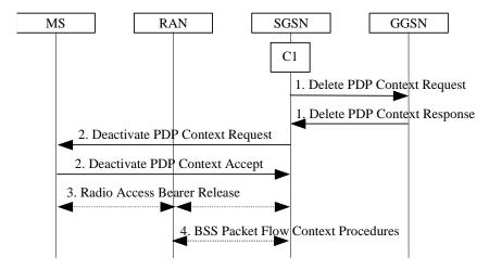
Figure 76: SGSN-initiated PDP Context Deactivation Procedure
