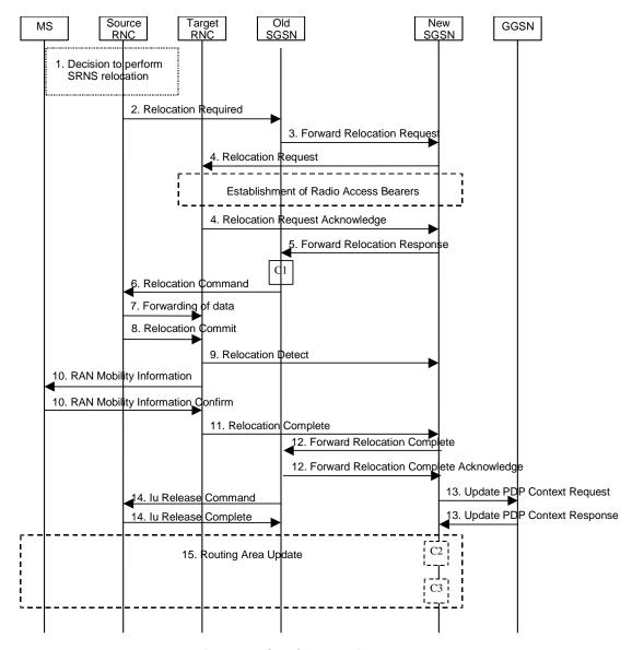
Figure 39: SRNS Relocation Procedure
