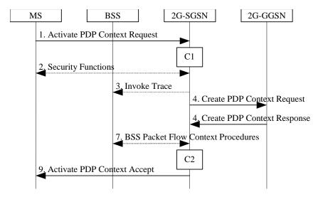
Figure 63: PDP Context Activation Procedure for GSM
