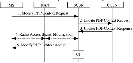
Figure 72: MS-Initiated PDP Context Modification Procedure
