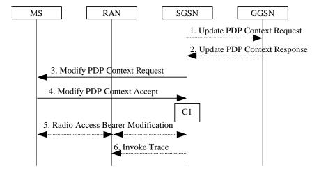
Figure 70: SGSN-Initiated PDP Context Modification Procedure
