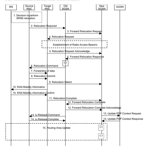
Figure 39: SRNS Relocation Procedure
