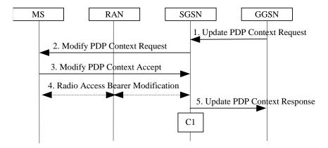
Figure 71: GGSN-Initiated PDP Context Modification Procedure
