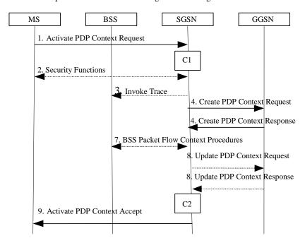
Figure 63: PDP Context Activation Procedure for A/Gb mode
