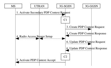
Figure 66: Secondary PDP Context Activation Procedure for UMTS
