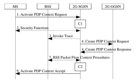
Figure 1: PDP Context Activation Procedure for GSM
