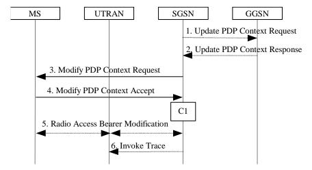
Figure 70: SGSN-Initiated PDP Context Modification Procedure
