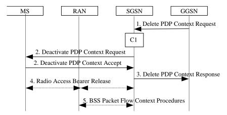
Figure 77: GGSN-initiated PDP Context Deactivation Procedure
