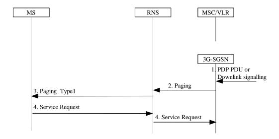
Figure 58: PS Paging Without RRC Connection for CS
