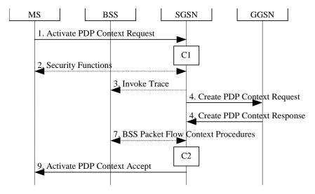
Figure 63: PDP Context Activation Procedure for A/Gb mode
