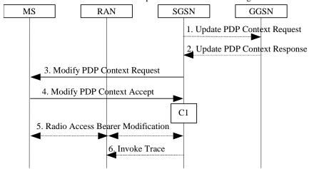
Figure 70: SGSN-Initiated PDP Context Modification Procedure
