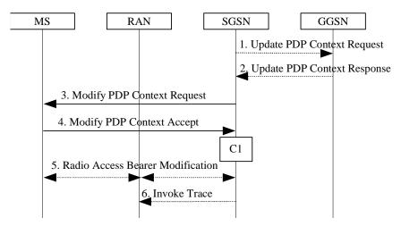
Figure 70: SGSN-Initiated PDP Context Modification Procedure
