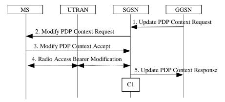
Figure 6: GGSN-Initiated PDP Context Modification Procedure
