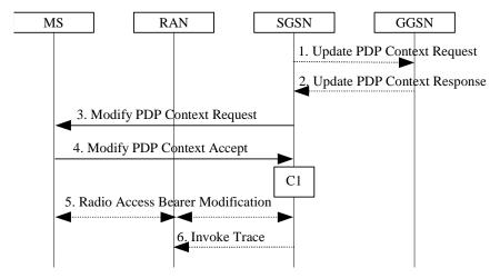
Figure 70: SGSN-Initiated PDP Context Modification Procedure
