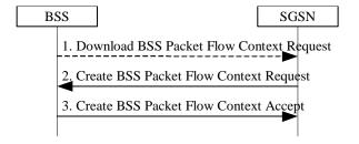
Figure 85: BSS Packet Flow Context Creation Procedure
