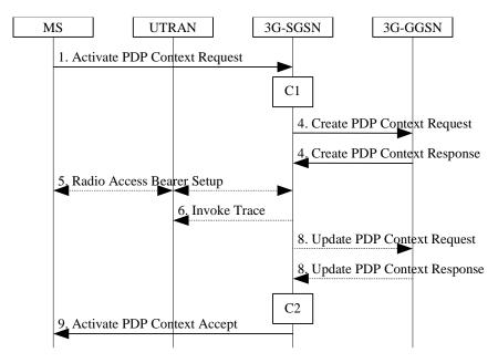
Figure 64: PDP Context Activation Procedure for UMTS
