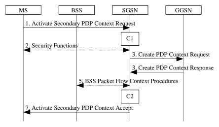
Figure 65: Secondary PDP Context Activation Procedure for A/Gb mode
