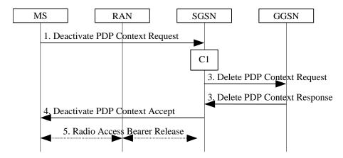
Figure 75: MS Initiated PDP Context Deactivation Procedure for lu mode
