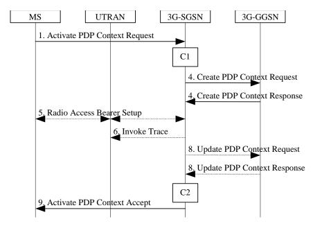
Figure 2: PDP Context Activation Procedure for UMTS
