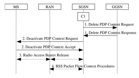
Figure 76: SGSN-initiated PDP Context Deactivation Procedure
