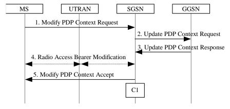
Figure 72: MS-Initiated PDP Context Modification Procedure
