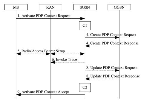
Figure 64: PDP Context Activation Procedure for Iu mode
