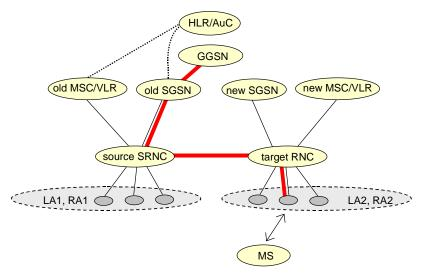
Figure 37: Before SRNS Relocation and Routeing Area Update
