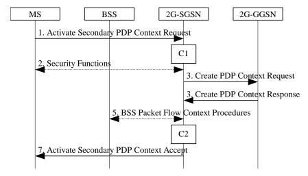
Figure 3: Secondary PDP Context Activation Procedure for GSM
