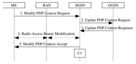
Figure 72: MS-Initiated PDP Context Modification Procedure
