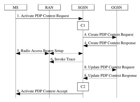
Figure 64: PDP Context Activation Procedure for lu mode
