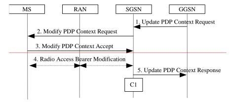
Figure 71b: GGSN-Initiated PDP Context Modification Procedure, lu mode
