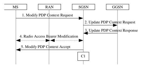
Figure 72: MS-Initiated PDP Context Modification Procedure
