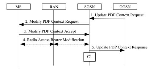
Figure 71: GGSN-Initiated PDP Context Modification Procedure
