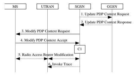
Figure 5: SGSN-Initiated PDP Context Modification Procedure
