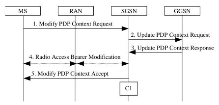
Figure 72: MS-Initiated PDP Context Modification Procedure
