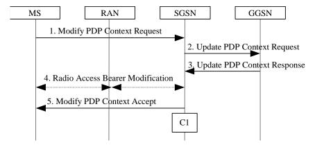
Figure 72: MS-Initiated PDP Context Modification Procedure
