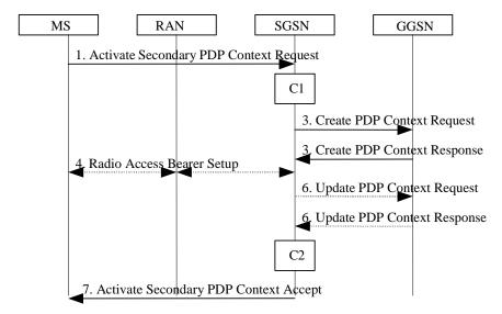
Figure 66: Secondary PDP Context Activation Procedure for lu mode
