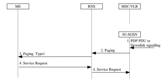
Figure 1: PS Paging Without RRC Connection for CS
