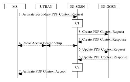
Figure 4: Secondary PDP Context Activation Procedure for UMTS
