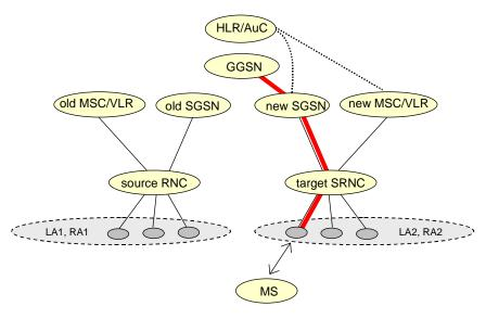
Figure 41: After Combined Hard Handover and SRNS Relocation and Routeing Area Update
