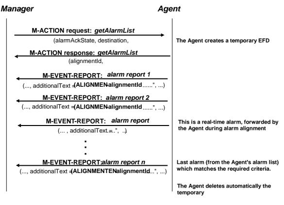
Figure 1: Alignment arrow diagram
