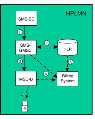
Figure 5.8: Delivery of a short message to a mobile subscriber
