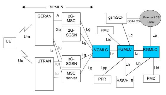
Figure 5.4: LCS logical architecture with inter-GMLC [Lr] interface
