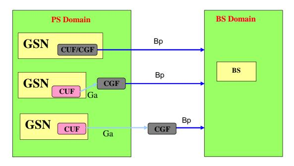
**GSN:** The core packet switching function (**G**PRS **S**upport **N**ode).
