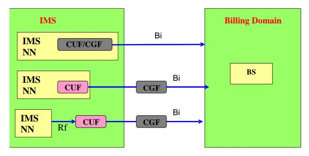
**IMS NN:** IP Multimedia subsystem network nodes include means P-, I- and S-CSCF, MRFC, MGCF, BGCF and the SIP based AS.
