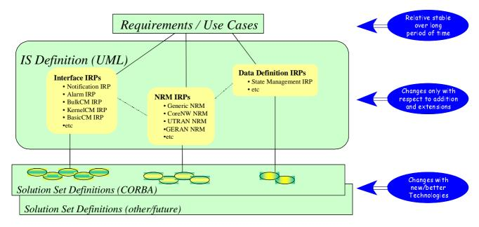
Figure 4.2: The IRP 3-Level Specifications Approach
