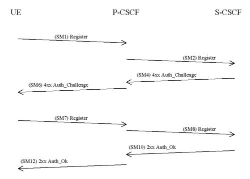
The UE sends a Register message towards the S-CSCF to register the location of the UE and to set-up the security mode, cf. clause 6.1. In order to start the security mode set-up procedure, the UE shall include a *Security-setup*-line in this message.
