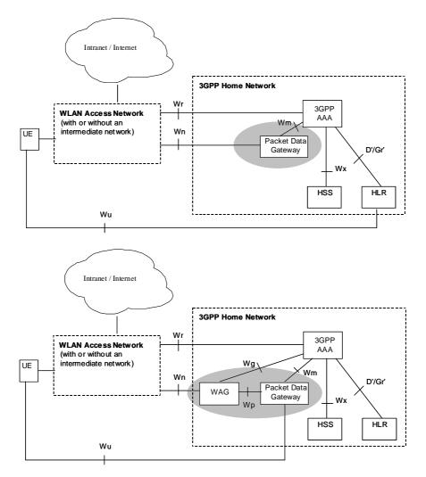
Figure 1: Non roaming reference model
