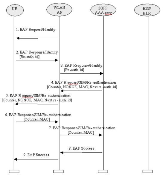
Figure 7: EAP SIM Re-authentication
