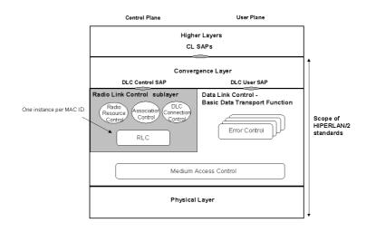
Figure A.5: Protocol stack in the MT
