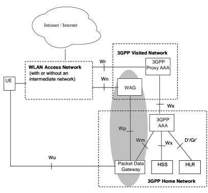
Figure 2: Roaming reference model, services in the HPLMN
