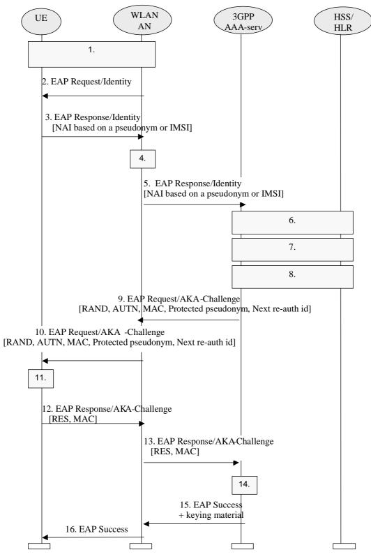
Figure 4: Authentication based on EAP AKA scheme
