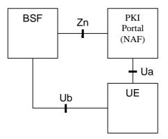
Figure 1: Simple network model for certificate issuing
