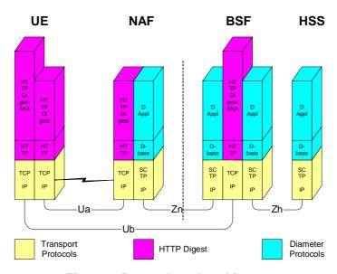
Figure 2: Protocol stack architecture
