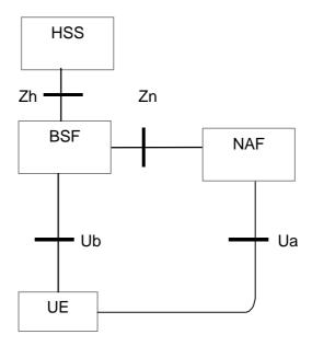
Figure 1: Simple network model for bootstrapping
