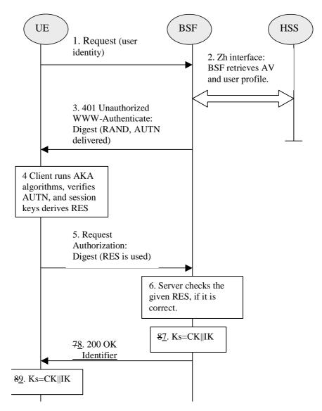
Figure 4: The bootstrapping procedure
