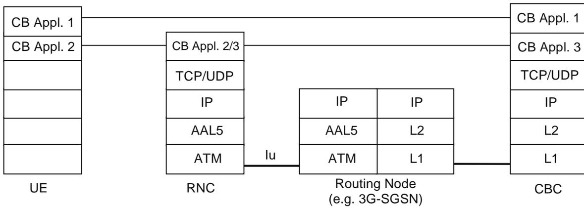
**Figure 4-47820: Common Communication Channel used by the Cell Broadcast Application Possible mapping of the Bc reference point onto the transport resources of the Iu interface**
