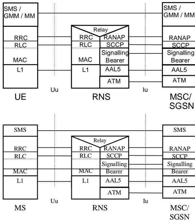
Figure 53 : Protocol architecture for 3G SMS for both a CS service domain and a PS service domain
