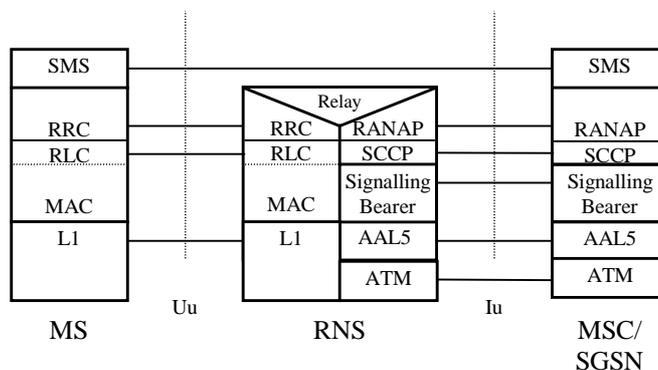
Figure 4-45: Protocol architecture for 3G SMS for both a CS service domain and a PS service domain
