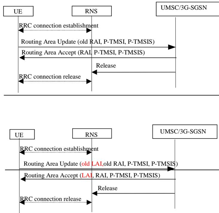
**Figure 25: Periodic update procedure when the MS is attached for both CS and PS services**
