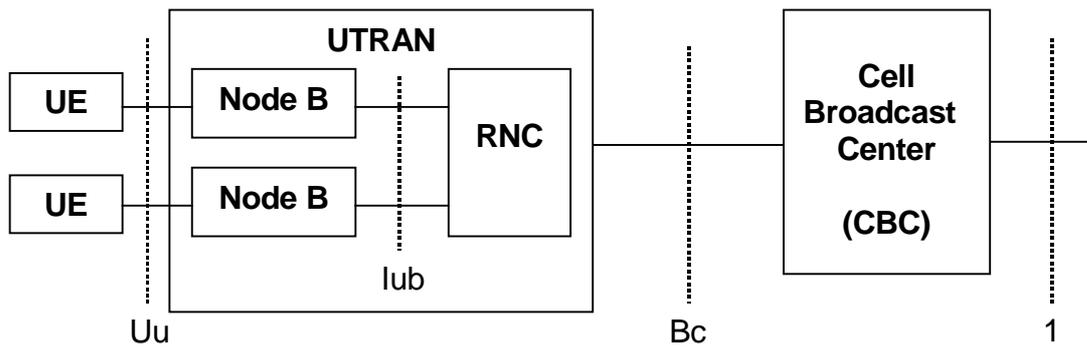
Figure- 4-46: Architecture for SMS-the Cell Broadcast Service in UMTS
