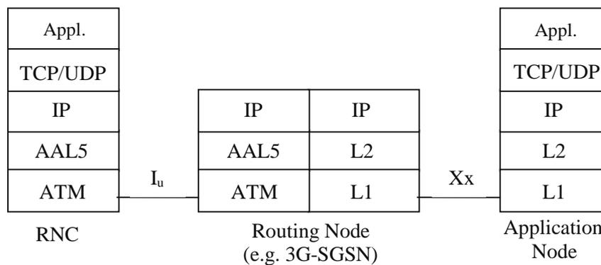
Figure 4 42: Protocol Stack of the Common Communication Channel
