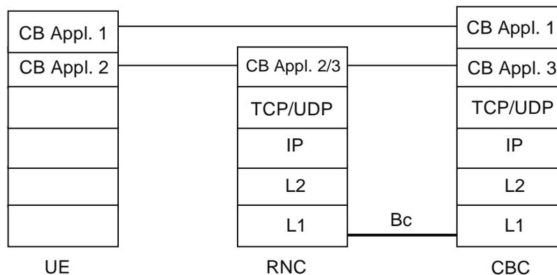
Figure 4-47: ~~Common Communication Channel used by the Protocol architecture for the Cell Broadcast~~
