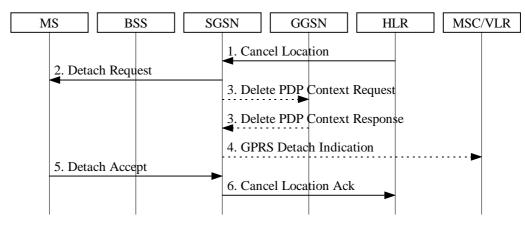
Figure 21: HLR-Initiated GPRS Detach Procedure
