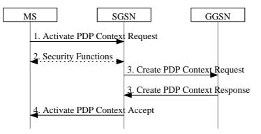
Figure 34: PDP Context Activation Procedure
