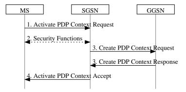
Figure 35: PDP Context Activation Procedure
