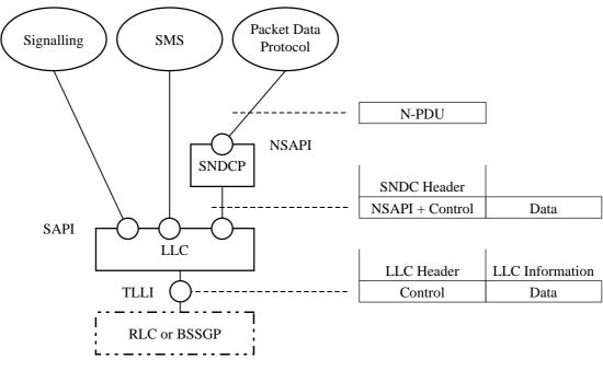
Figure 46: Multiplexing of Network Protocols
