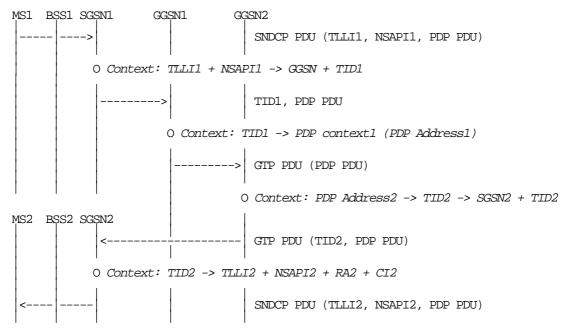
Figure C.4: MS-to-MS Data Routeing via Different GGSNs
