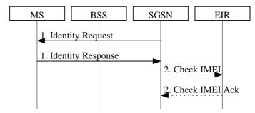
Figure 26: Identity Check Procedure
