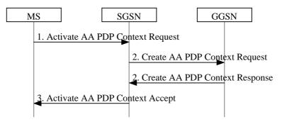
Figure 38: Anonymous Access PDP Context Activation Procedure
