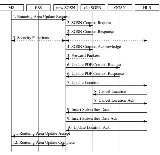
Figure 28: Inter SGSN Routeing Area Update Procedure
