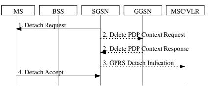
Figure 19: SGSN-Initiated GPRS Detach Procedure
