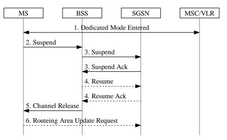
Figure 54: Suspend and Resume Procedure
