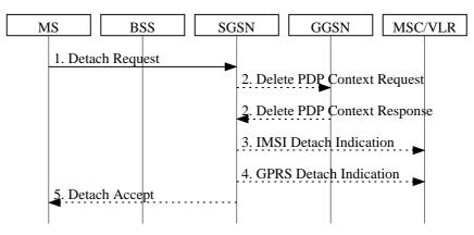
Figure 19: MS-Initiated Combined GPRS / IMSI Detach Procedure
