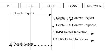
Figure 18: MS-Initiated Combined GPRS / IMSI Detach Procedure
