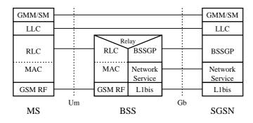
Figure 5: Signalling Plane MS - SGSN
