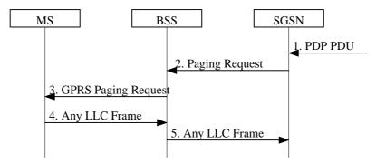
Figure 32: GPRS Paging Procedure
