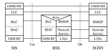
Figure 5: Signalling Plane MS - SGSN
