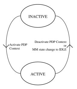
Figure 33: Functional PDP State Model
