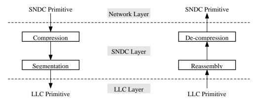
Figure 46: Sequential Invocation of SNDC Functionality
