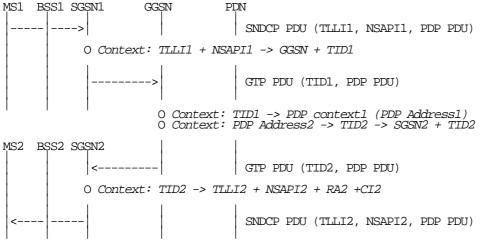
Figure C.3: MS-to-MS Data Routeing via the Same GGSN
