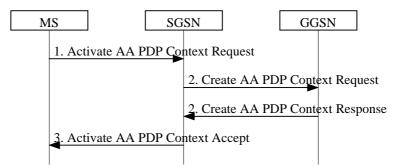
Figure 39: Anonymous Access PDP Context Activation Procedure
