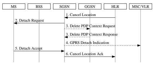
Figure 20: HLR-Initiated GPRS Detach Procedure
