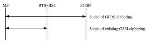
Figure 24: Scope of GPRS Ciphering
