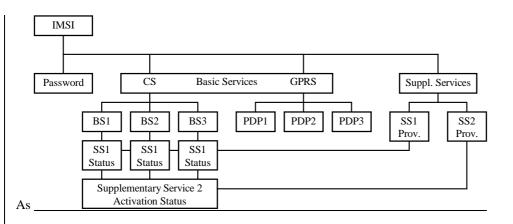
Figure 52 indicates, the GPRS subscription data is at the same level as basic services. Each PDP subscription is seen as a basic service. Supplementary services are provisioned as part of the overall subscription. Activation of SSs is either at the basic service level (SS1) or at the <u>PDPoverall</u> subscription level (SS2).
