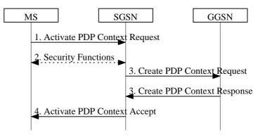
Figure 1: PDP Context Activation Procedure
