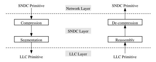
Figure 47: Sequential Invocation of SNDC Functionality
