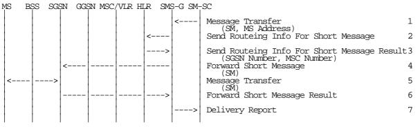
Figure 51: MT SMS Transfer, Successful
