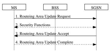
Figure 2: Intra SGSN Routeing Area Update Procedure
