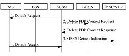
Figure 20: SGSN-Initiated GPRS Detach Procedure
