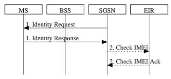
Figure 25: Identity Check Procedure
