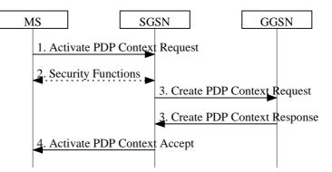
Figure 1: PDP Context Activation Procedure
