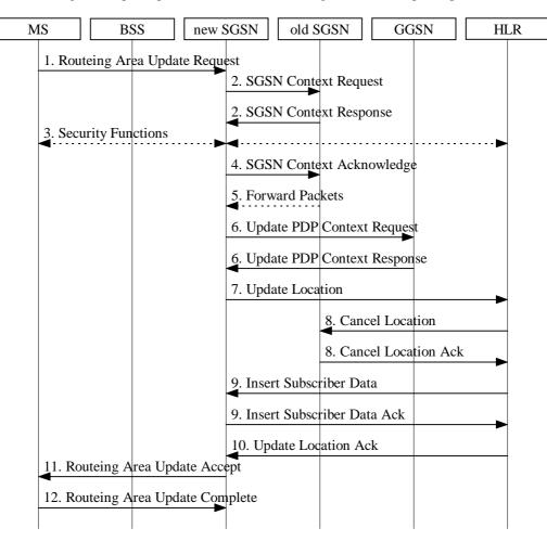
Figure 3: Inter SGSN Routeing Area Update Procedure
