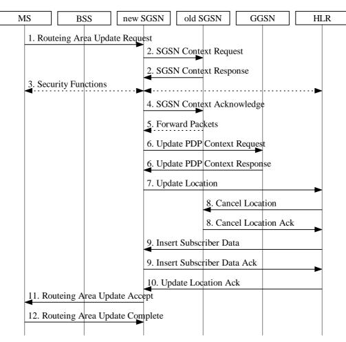
Figure 27: Inter SGSN Routeing Area Update Procedure
