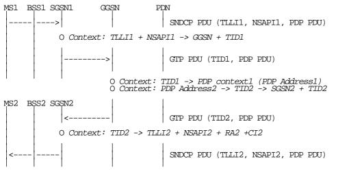
Figure B.3: MS-to-MS Data Routeing via the Same GGSN
