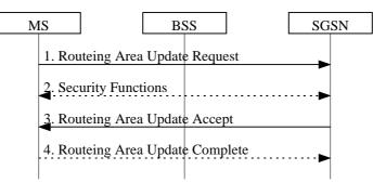
Figure 26: Intra SGSN Routeing Area Update Procedure
