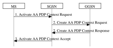
Figure 2: Anonymous Access PDP Context Activation Procedure
