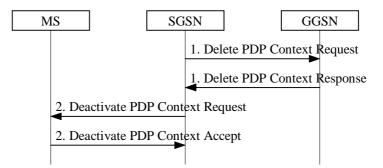
Figure 42: PDP Context Deactivation Initiated by SGSN Procedure
