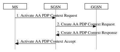
Figure 2: Anonymous Access PDP Context Activation Procedure
