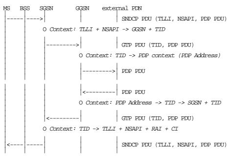
Figure B.1: Data Routeing in HPLMN to and from an External PDN
