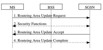
Figure 27: Intra SGSN Routeing Area Update Procedure
