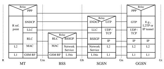
Figure 49: Transmission Plane for PDP Type PPP
