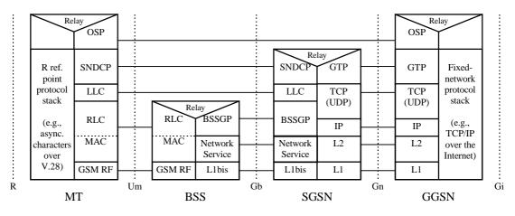
Figure 48: Relationship of OSP to the Rest of the GPRS Protocol Architecture
