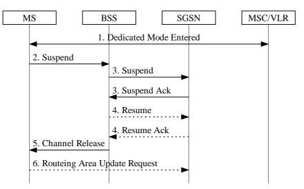
Figure 58: Suspend and Resume Procedure
