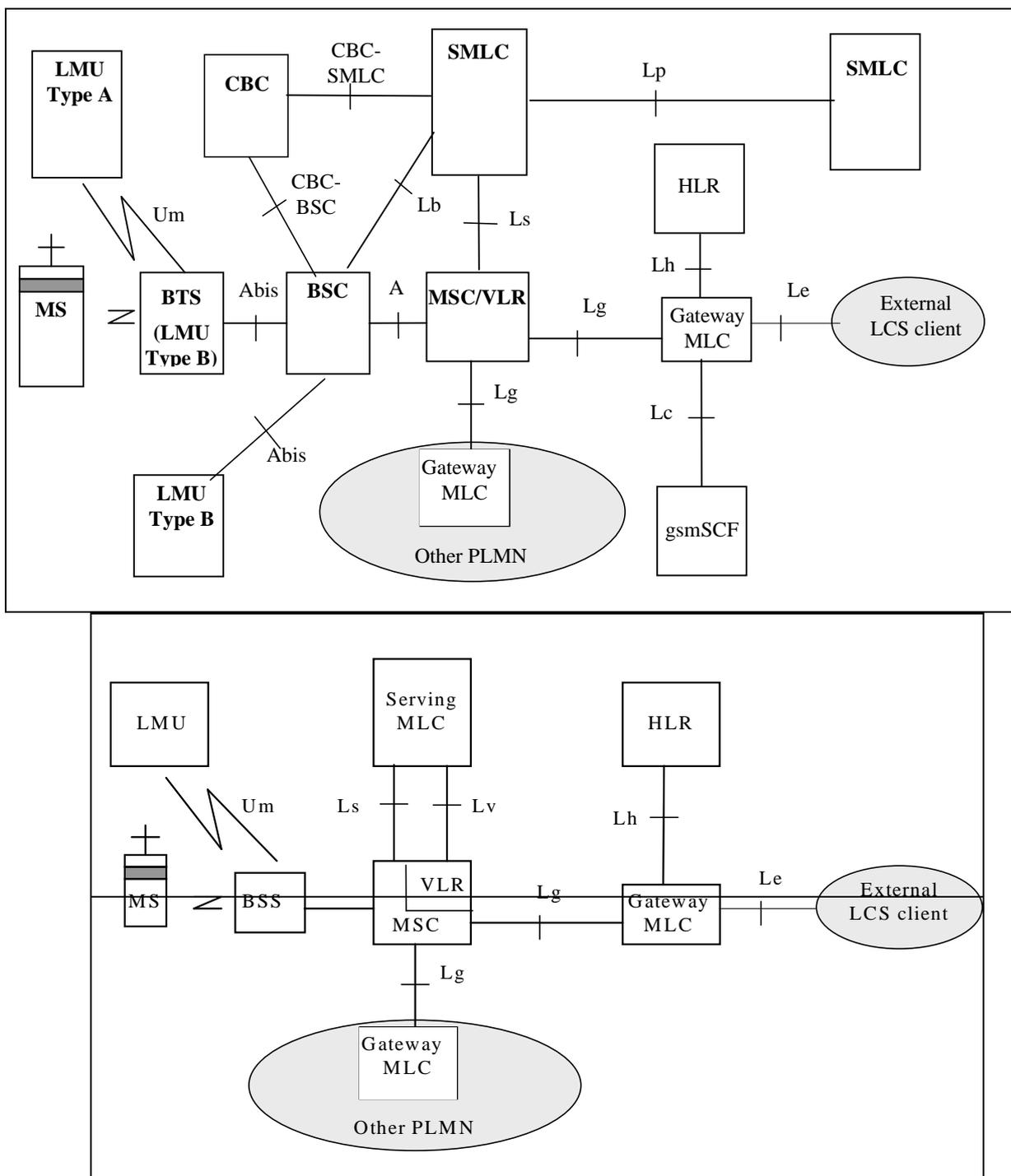
Figure 4: Configuration of a PLMN supporting LCS
