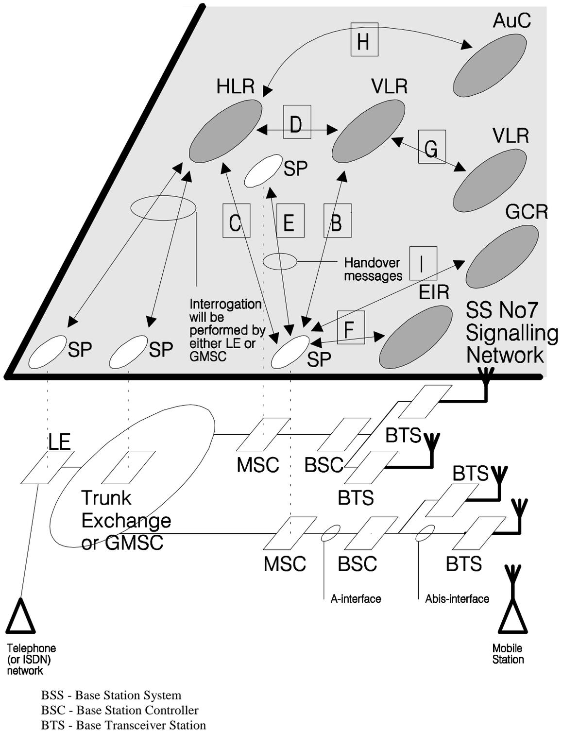
Figure 1: Configuration of a PLMN (not supporting GPRS) and interfaces
