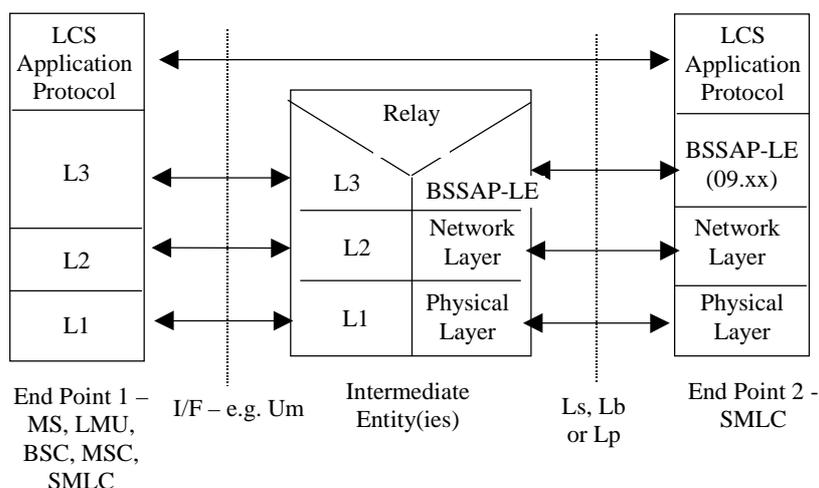
**Figure 1** – Generic Model for LCS Signaling to an SMLC
