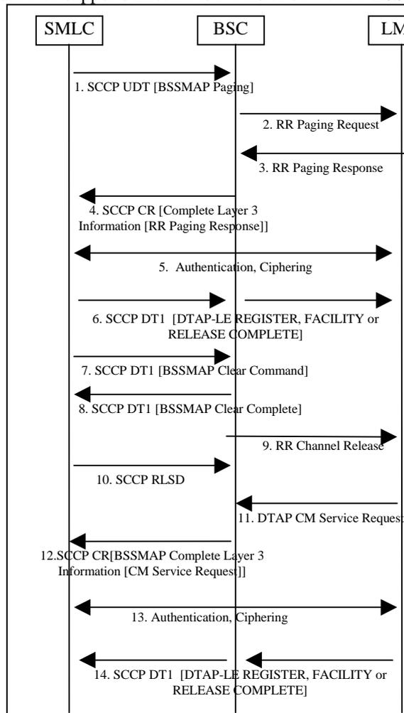
**Figure 31 Information Transfer between a BSS based SMLC and a Type A LMU**
