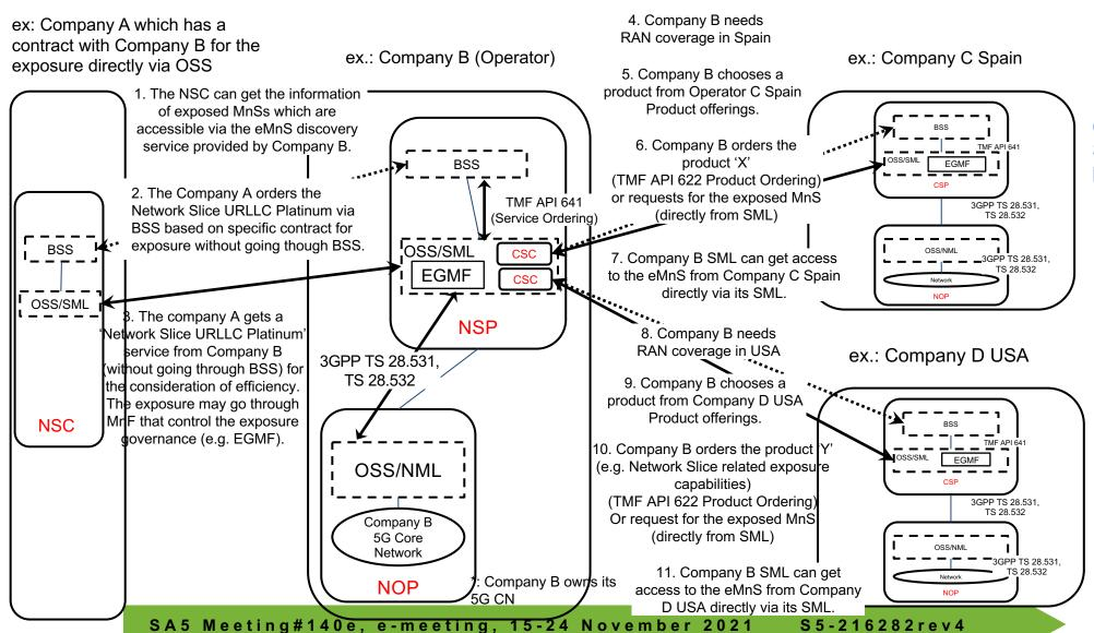
CSC connecting to Operator C Spain and Operator D USA belongs to SML.
