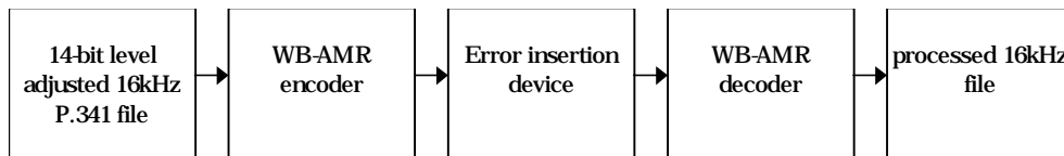
Figure 5: Processing of WB-AMR conditions.
