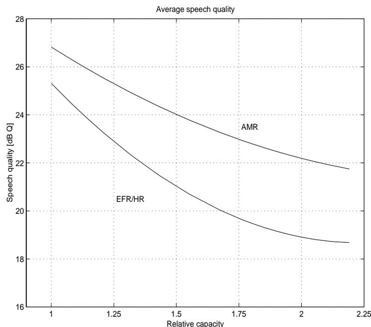
Fig. 6.1 - Average speech quality vs. relative capacity for AMR and EFR/HR
