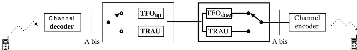
Fig. 6.4 - Mobile to mobile communication link.
