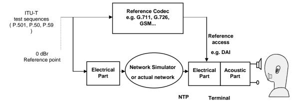
Fig. 3: Test setup for terminals, electrical access using a "reference" access or a network simulator
