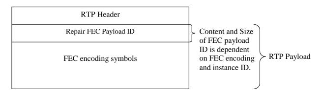
Figure 13: RTP payload structure for repair RTP packets
