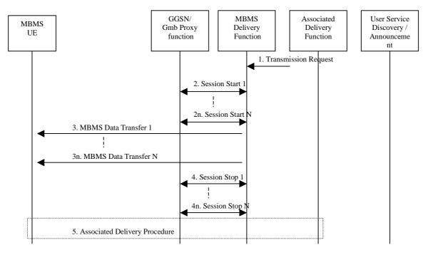
Figure 8: Procedure of MBMS Data Transfer
