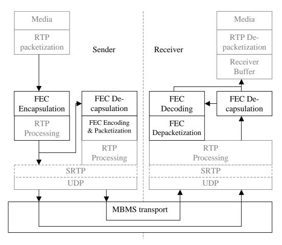
Figure 11: FEC mechanism for RTP interaction diagram
