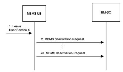
Figure 7: Termination of an MBMS user service
