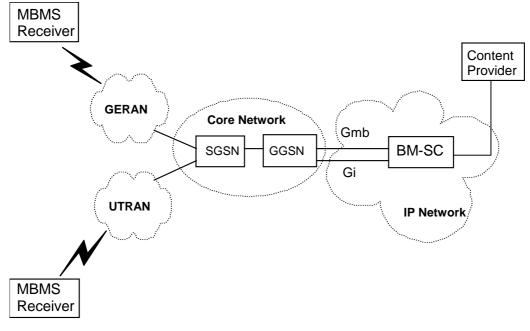
Figure 3 MBMS network architecture model
