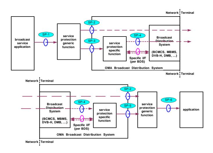
**Figure 5: Service Protection Function Architecture**
