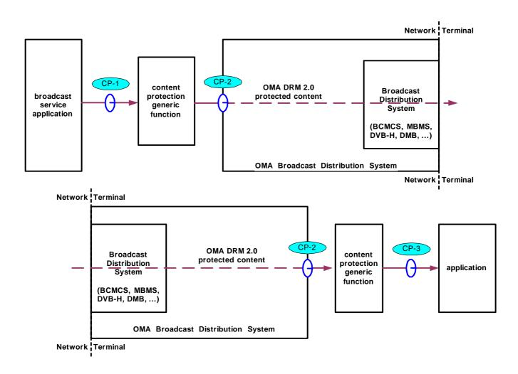
**Figure 6: Content Protection Function Architecture**
