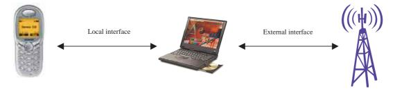
The mobile phone (the "card holding device") on the left holds the UICC or SIM (the "card") and the laptop holds the functions for WLAN access (the "WLAN access device"). The network is not aware of the UE functional split. Typically the card holding device also has a network interface (although not necessarily WLAN interface), e.g. a GSM or UTRAN interface.
