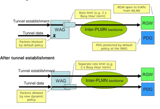
In summary, the PDG is protected from 'unauthorised' traffic from the WLAN until after Tunnel Establishment. It has been suggested that this results in less stringent robustness requirements on the PDG and is therefore a security advantage.
