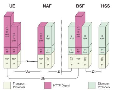
Figure 2: Protocol stack architecture
