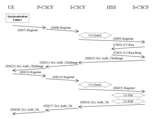
The flow equals the flow in 6.1.1 up to SM6. When the UE receives SM6 it detects that the SQN is out of range and sends a synchronization failure back to the S-CSCF in SM7. Draft-ietf-sip-digest-aka-01 [17] describes the fields to populate corresponding parameters of synchronization failure.
