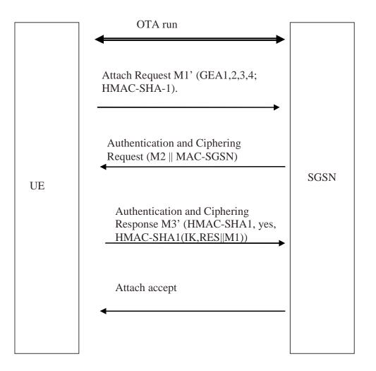
Whereby M1, M2 and M3 are the messages as known from current specifications (See TS 24.008). The three way handshake is kept but the message content (M1',M2',M3') is changed and additional algorithm support is required at both terminal and SGSN.
