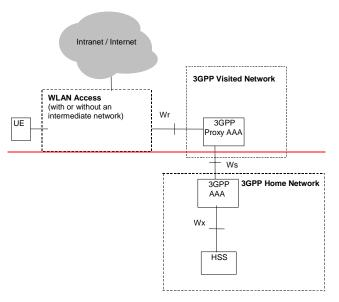
Figure 4.1: Access Control Reference Model
