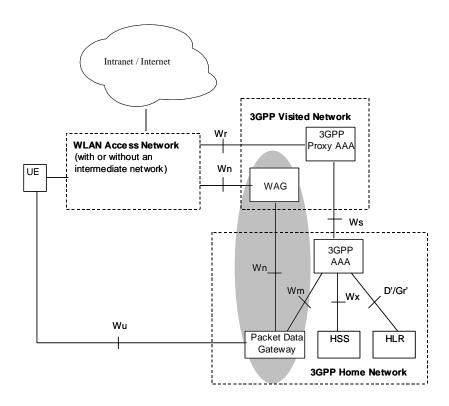
Figure 4.2 Roaming reference model, services in the HPLMN
