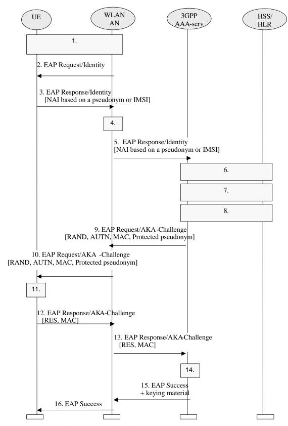
Figure 7.1: Authentication based on EAP AKA scheme
