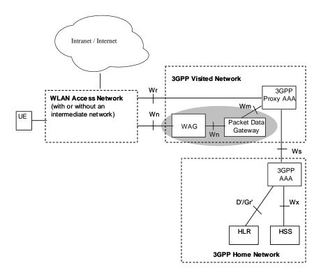
Figure 4.3 Roaming reference model, services in the VPLMN
