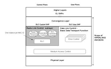
Figure A.5: Protocol stack in the MT
