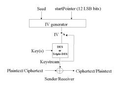
Figure A.7: The encryption/decryption function
