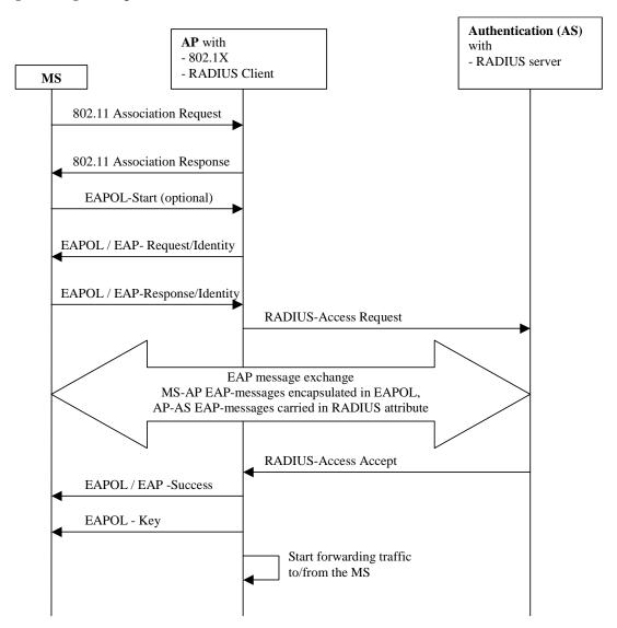
Figure A.3: General EAP authentication with 802.11i and RADIUS as AAA protocol
