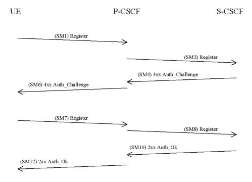
The UE sends a Register message towards the S-CSCF to register the location of the UE and to set-up the security mode, cf. section 6.1. In order to start the security mode set-up procedure the UE shall include a *Security-setup-line* in this message. The *Security-setup-line* in SM1 contains the SPIs and the numbers of the protected ports assigned by the UE for the SAs for TCP and UDP. It also contains a list of identifiers for the integrity algorithms which the UE supports.
