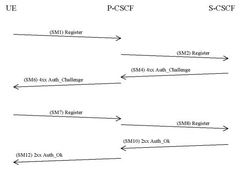
The UE sends a Register message towards the S-CSCF to register the location of the UE and to set-up the security mode, cf. clause 6.1. In order to start the security mode set-up procedure, the UE shall include a *Security-setup*-line in this message. The *Security-setup-line* in SM1 contains the SPIs and the numbers and of the protected ports assigned selected by the UE for the SAs for TCP and UDP. It also contains a list of identifiers for the integrity algorithms which the UE supports.
