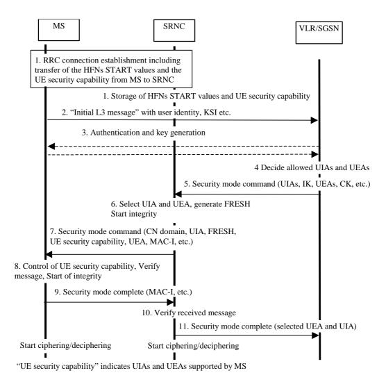
Figure 14: Local authentication and connection set-up
