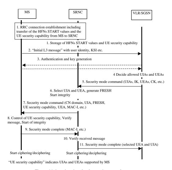
Figure 14: Local authentication and connection set-up
