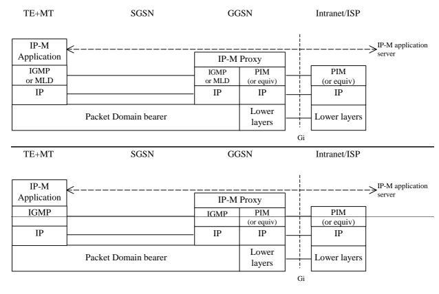
Figure 12: Protocol configuration for IP-Multicast handling (control plane)
