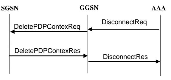
Figure 25: PDP Context deletion with RADIUS
