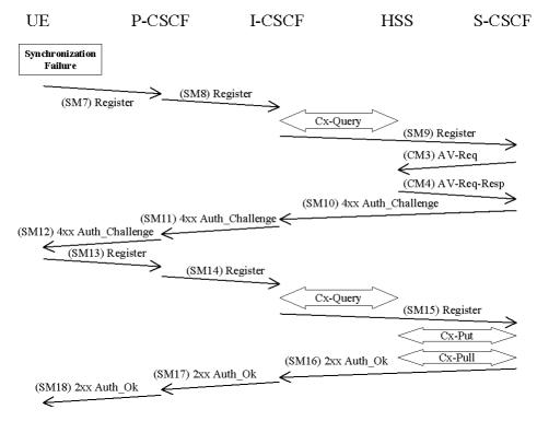
The flow equals the flow in 6.1.1 up to SM6. When the UE receives SM6 it detects that the SQN is out of range and sends a synchronization failure back to the S-CSCF in SM7.
