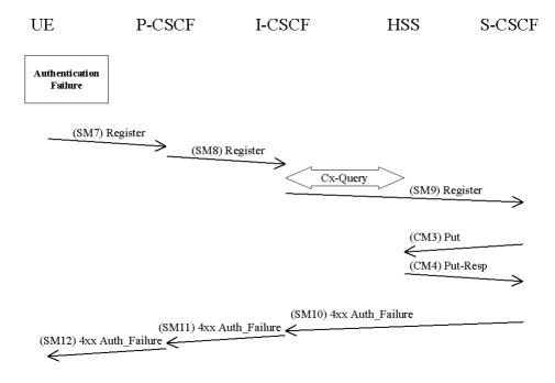
The UE shall send a Register message towards the HN including an indication of the cause of failure in SM7. The P-CSCF and the I-CSCF forward this message to the S-CSCF.
