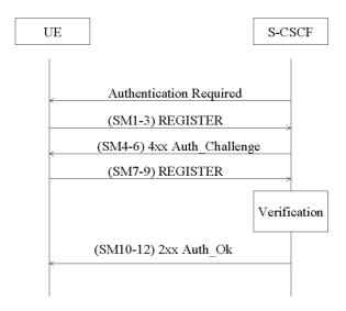
The UE shall initiate the re-registration on the reception of the Authentication Required indication. In the event that the UE does not initiate the re-registration procedure after the request from the S-CSCF, the S-CSCF may decide to deregister the subscriber or re-issue an Authentication-Required.
