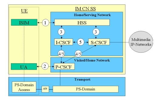
Figure 1: The IMS security architecture
