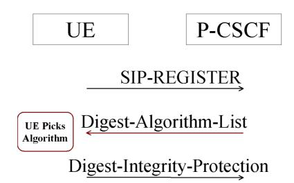
This security mode set-up looks different to the current requirements defined in clause 7 where the P-CSCF chooses the algorithm. A proposed mechanism for bidding down protection is to utilise a nonce, which will have a meaning for the client. The nonce-value in this case is not longer only a random number it will include the integrity algorithm and quality of protection along with the traditional nonce value. The nonce in this case could look like:
