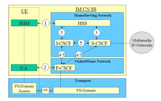
Figure 1. The IMS security architecture
