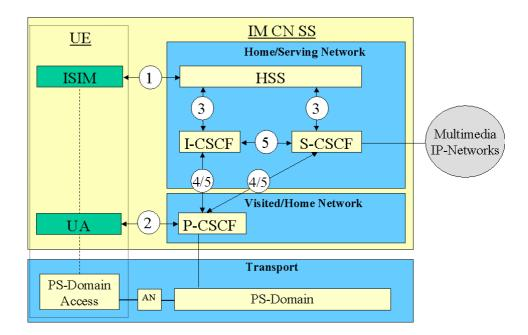
Figure 1. The IMS security architecture
